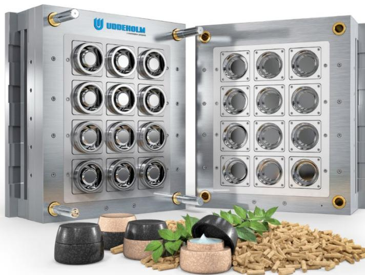
Bio-composites can often cause a combination of both wear and corrosion, due to wood fibres and water vapour. This failure mode is also known as tribochemical wear.
